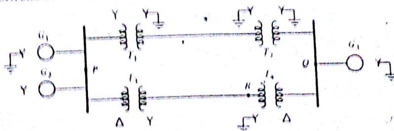
Suppose loads driving critical processes are connected at P, Q and R. What precautions should be taken so that these loads are not disrupted by the occurrence of an LG fault anywhere on the network?
